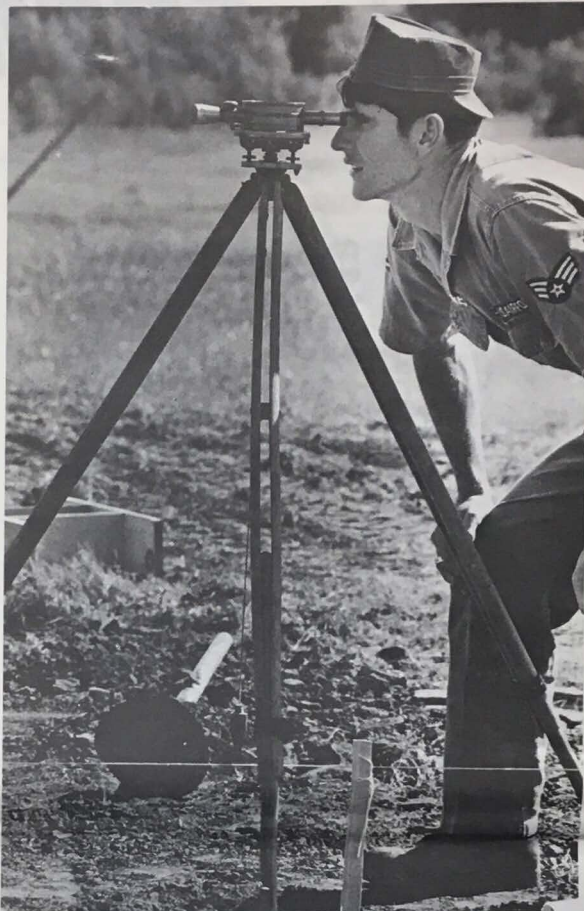
Sgt. James Ecker takes a long look through his surveying level.
